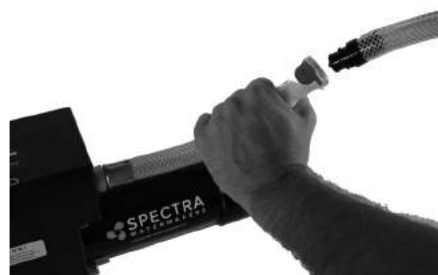
Connecting brine discharge service-hose
