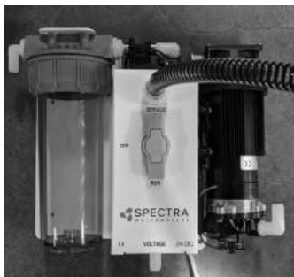
Service hose connected and service valve to SERVICE
